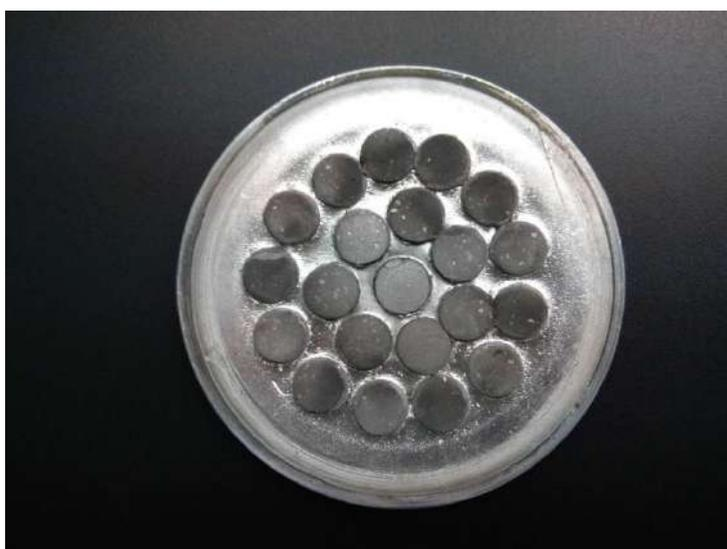
**Fig.1.** View of the target, consisting of a matrix and 21 disks.
