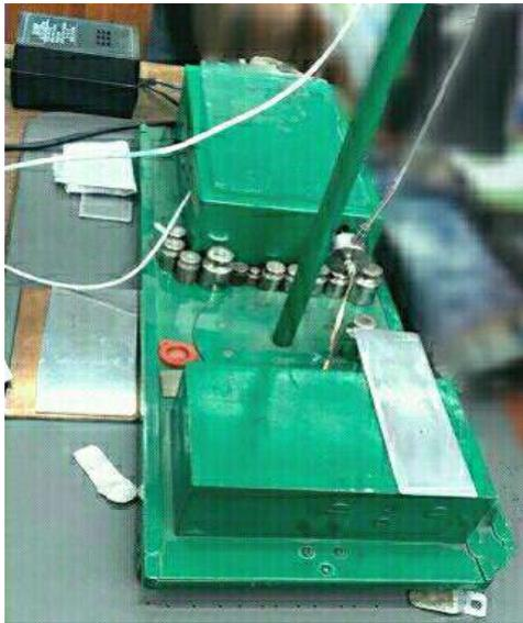
**Fig.2.** Information - measuring device for determining the coefficient of sliding friction.
