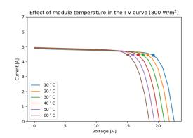
Fig.6. Simulation results of dependence between voltage and current at different temperatures
