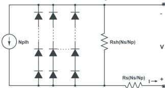
Fig.8. The electrical circuit of the solar panel.
