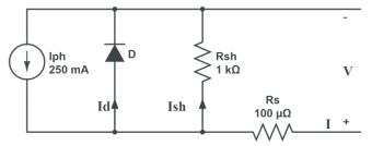
Fig.3. The electrical circuit of the photocell.
