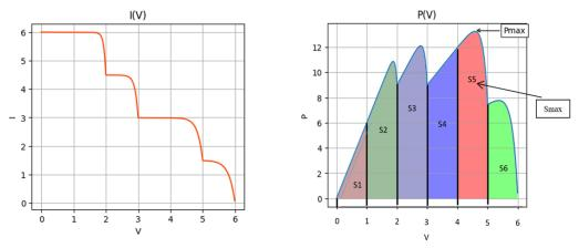
Fig. 17. MPPT algorithm in case of darkening or loss of an element/elements
