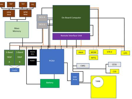
Fig.1. Electrical architecture of the KazEOSat -1.
