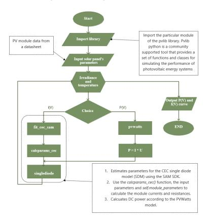
Fig.4. The python code algorithm for solar panels in the form of the diagram
